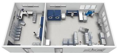
Installed between two separate area, avoids all contact between dirty (infectious) linen and the clean linen, and any type of re-contamination during the process.
